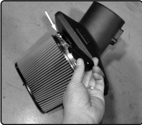
**13.** Place the filter onto the Injen plenum and then secure the clamp
