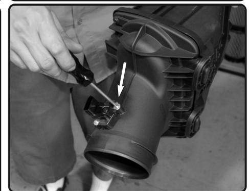
**8.** Loosen the 2 screws holding in the MAF sensor, remove the sensor.
