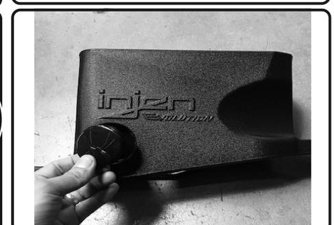
**12.** Install the Filter Minder plug into the Filter Minder hole located on top of the air box assembly.
