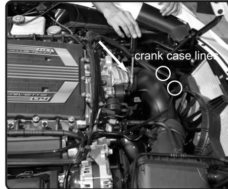
**3.** Loosen the clamps on the stock intake tube using 8mm nut driver. Disconnect the crank case lines on intake tube.
