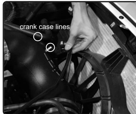
**22.** Reconnect both crank case fittings. Some models only have 1 crank case line. Remove the fitting and use the supplied 3/8"-16 Hex bolt to block the fitting if not used. Secure threads with Loctite
