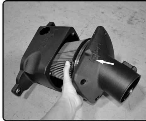
**14.** Install the plenum assembly into the lower air box.
