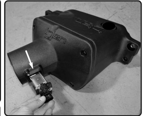
**16.** Now install the MAF sensor into the plenum. Secure using provided M4 screws.
