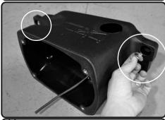
**11.** Now install the grommets and washer-spacers to the new injen airbox.
