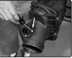
**8.** Loosen the 2 screws holding in the MAF sensor, remove the sensor.
