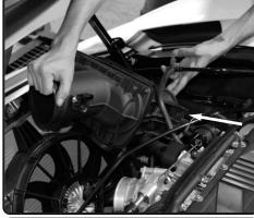
**7.** Carefully remove the air box out of the vehicle.
