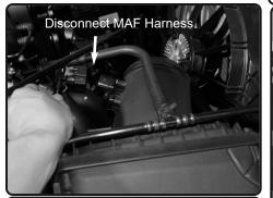
**5.** Pull back lines away from the air box. Disconnect MAF sensor harness.
