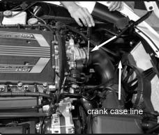
**3.** Loosen the clamps on the stock intake tube using 8mm nut driver.. Disconnect the crank case line on intake tube.
