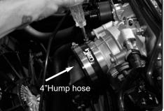
**9.** Install the 4" hump hose with clamps to throttle body. Tighten the clamp on throttle body only.
