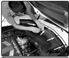
**2.** Use a 7mm nut driver to remove the four air vent screws. Remove the air vent from the engine bay for now.
