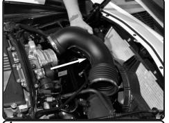
**4.** Now pull out the intake tube out of vehicle.
