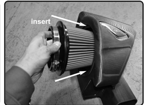
8. Install the filter into the passenger side air box housing. Position the Twist-Lock™ filter pattern to the hole cut out on air box.
