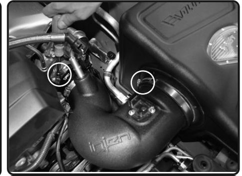
**16.** Adjust if needed, secure and tighten the clamp on turbo using 8mm nut driver. Tighten clamp on filter also.
