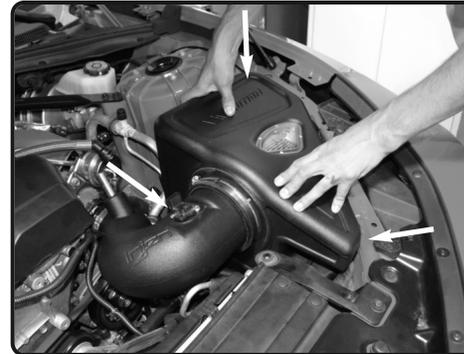
**15.** Make sure the intake tube is secured on the turbo. Make sure the airbox is seated properly. Position for best fit.
