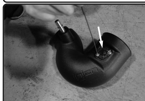
11. Secure and tighten the MAF sensor using provided M4 button head screws.
