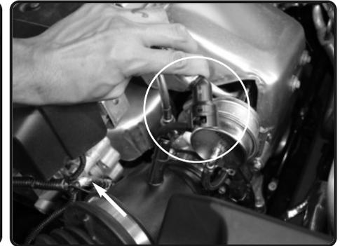
4. Now disconnect the Crank case fitting from the intake tube and pull back from tube.
