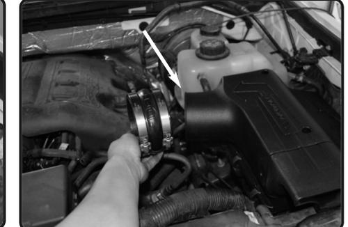
**8.** Place the 4.00" hump hose and 2-#64 clamps onto the Injen intake plenum. Make sure you push the hump hose all the way over to allow room for the intake tube.
