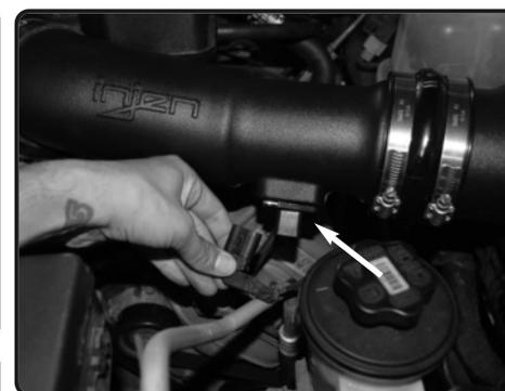
**10.** Install the MAF sensor and 2-M4 bolts to secure the MAF sensor to the Injen intake tube. Re-connect the MAF harness.
