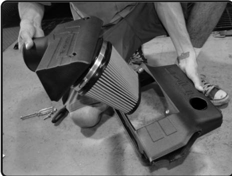
**5.** Once the Filter Minder plug is installed in the upper air box, install the filter onto the Injen air box plenum.
