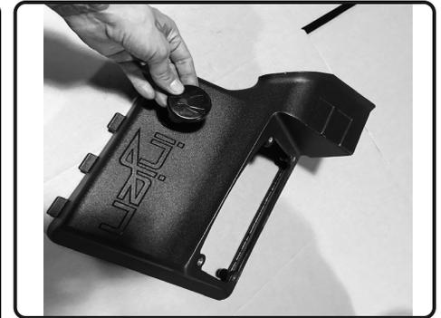
**4.** Place the Filter Minder plug into the hole on the upper air box assembly
