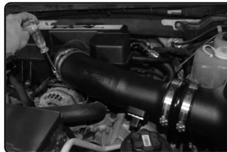
**9.** Install a 4.00" straight hose and 2-#64 clamps onto the OE air box resonator and then install the Injen intake tube. Adjust the intake pipe for best fitment and then secure all the clamps.
