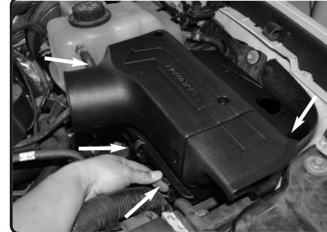
**7.** Install the Injen upper airbox and plenum onto the lower OEM airbox assembly and attach the 3 factory metal clips to secure the Injen air box to the OEM air box
