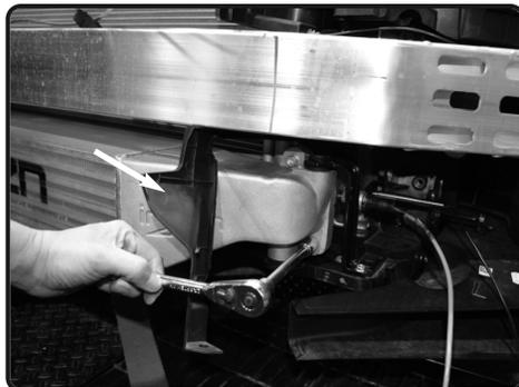
**21.** Tighten the Passenger and driver side intercooler using 12mm socket or wrench.
