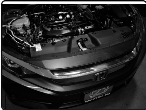
1. Remove the plastic rivet clips to remove the radiator support cover.
