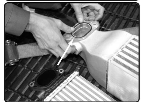
11. Now Remove the OEM gasket from the stock intercooler on both sides.
