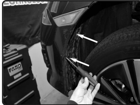
7. Carefully raise the vehicle up and unscrew the 2 screws on both sides of bumper.
