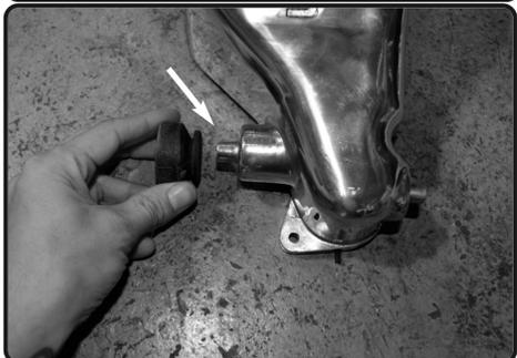
**20.** Install the grommet to the injen intercooler fitting.
