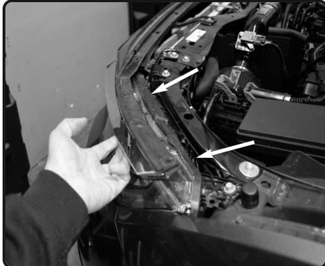
5. With flat head screwdriver, locate the push clip and pull back the top of the headlight trim. **Carefull not pull to hard.**
