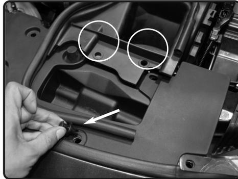
2. Loosen the screws holding in the ram scoop. pull back the Ram scoop from the intake.
