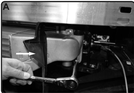
**20.** Re-install the OEM screws and secure the Injen intercooler.
