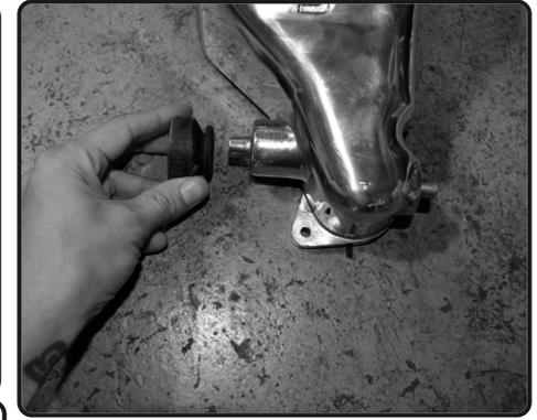
**19.** Install the grommet to the injen intercooler fitting.
