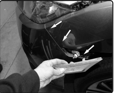
4. With flat head screwdriver carefully push clip back, and remove the side indicator. Pull panel of bumper back.
