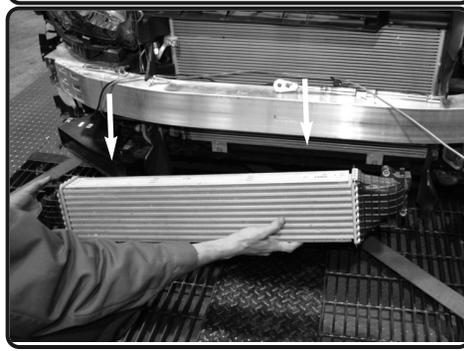
10. Now carefully pull out the intercooler from the vehicle.
