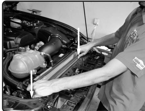
**18.** Locate and detach the two plastic locking tabs on each side of the AC condenser. This will allow you to lift the AC condensor up 1" to allow removal of the OE intercooler
