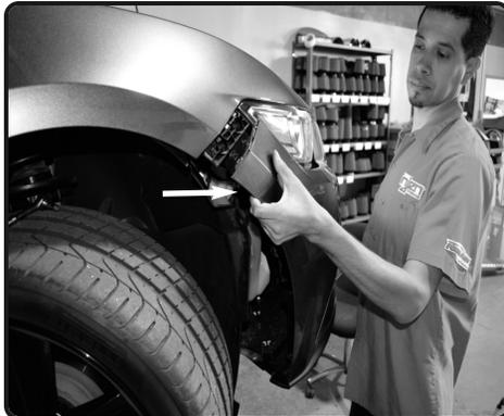
**5.** Once you have removed the screws from figure 4, carefully pull out on the side of the bumper to detach the front bumper from the bumper bracket.
