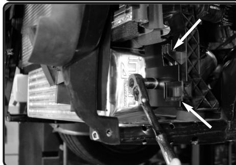
**22.** Slide the supplied #20122 bracket onto the left factory intercooler support tabs and then attach the intercooler with a M8 bolt and washer. Leave the bolt loose for now.
