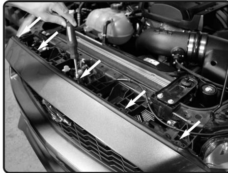
**2.** Remove the 5 - 8mm screws on top of the bumper.
