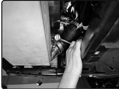
**21.** Reconnect both OE charge hoses to the Injen intercooler and then secure the clamps.
