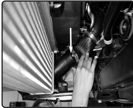
**17.** Loosen the clamp and detach the OE charge hose from the OE intercooler on the right side.
