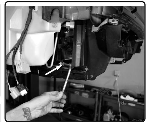
**15.** Remove the 10mm bolt from the front left side of the OE intercooler.
