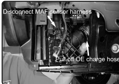
**14.** From the drivers side, disconnect the MAF sensor harness from the OE intercooler. Then loosen the clamp on the OE charge hose and pull the hose from the OE intercooler.
