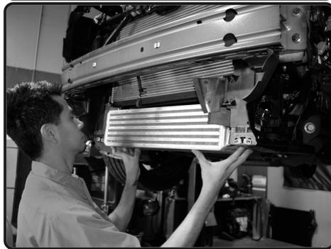
**21.** Place the Injen Intercooler into position. You may need an assistant to hold the intercooler while you place the brackets.
