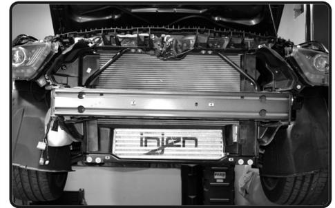
**23.** Your Injen intercooler installation is now complete. Make your final adjustment and make sure all your nuts, bolts and clamps are secure. Reinstall the rest of the bumper components in reverse order.
