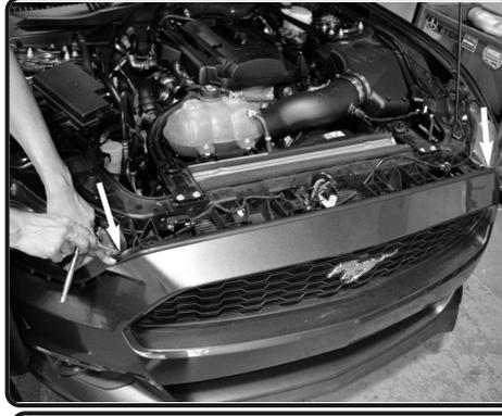
**6.** Remove the last 5.5mm screws from the front bumper located at the top on the ends of the bumper near the headlight.
