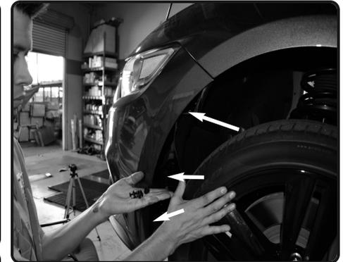
**3.** Remove the 3 plastic rivet clips from the side of the bumper on the wheel well cover. Repeat for the other side.
