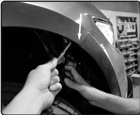
**4.** Pull back on the wheel well cover to access the 7mm screw holding the bumper to the fender in place. Repeat for the other side.
