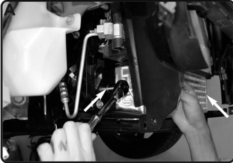
**20.** Make your final adjustment on the Injen intercooler for best fitment and then secure both the 8mm bolts on the brackets to secure the intercooler.
