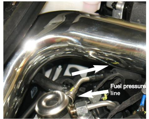
15. **CAUTION:** Make sure the bottom of the intake pipe does not rub on the high pressure fuel line. This line is connected to the fuel pressure regulator indicated in the photo.
