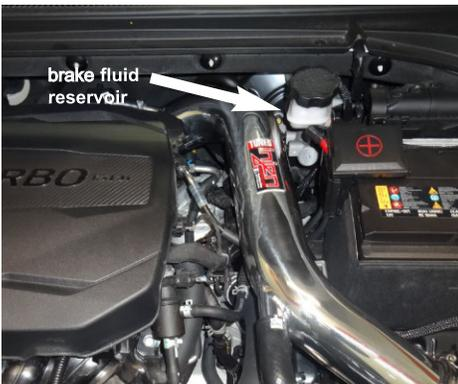
16. **CAUTION:** Make sure the intake pipe has adequate clearance from the brake fluid reservoir. Adjust the intake pipe for best possible fitment and then secure the all the clamps.
