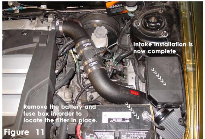
**Note: Removal of the battery and fuse box will be required before starting this installation.**
