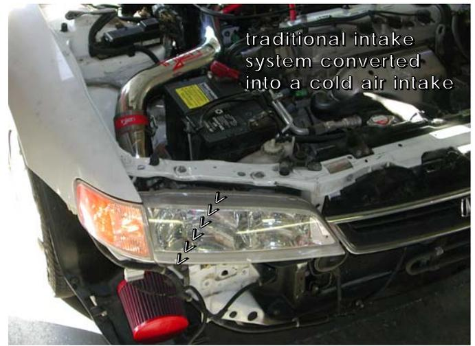
**Note: Disconnect the negative battery terminal before starting this installation.**
