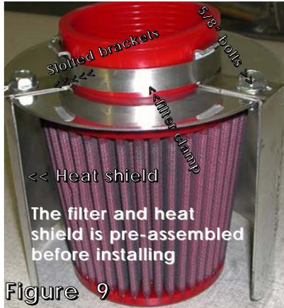
Slotted brackets >>>> 5/8" bolts >>>> Filter clamp >>>> <<< Heat shield
