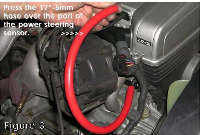
Press the 17"-6mm hose over the port of the power steering sensor. >>>>
