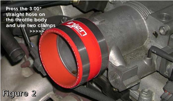
Press the 3.00" straight hose on the throttle body and use two clamps >>>>
