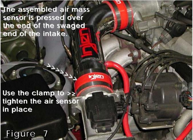
The assembled air mass sensor is pressed over the end of the swaged end of the intake.
