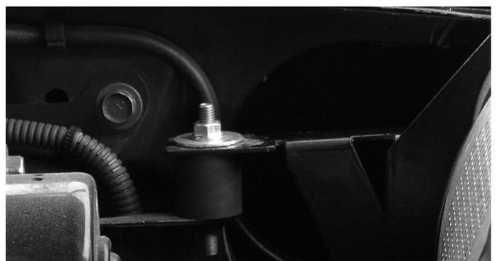
Here is a side view of the Power box bracket connected to the vibra-mount stud.
