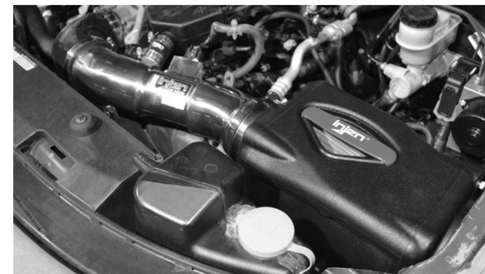
Congratulations! You have just completed the installation of the World's first tuned intake system, the Power-Flow intake, featuring MR Technology. Periodically, check the system for fitment, this will enhance the life of your Power-Flow system.
