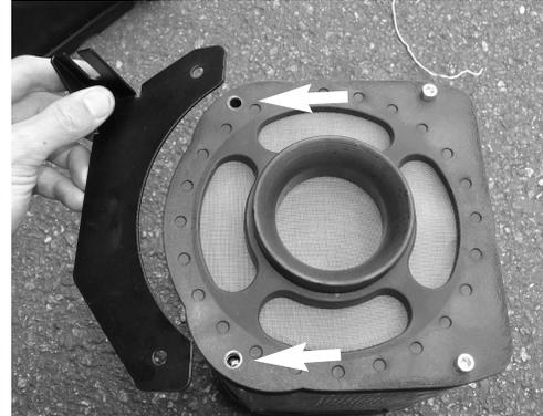
Secure the bracket to the PowerFlow box using provided M6 screws. Then align the mounting bracket onto this location.
