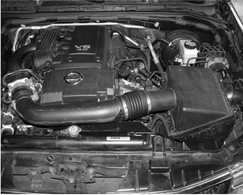
Picture of factory air intake system
