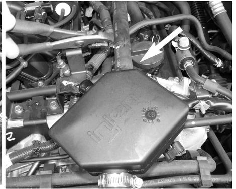
Insert crank case breather line over CCV box port and use stock clamp to secure breather line.
