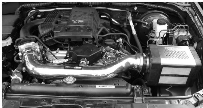
Check the alignment and fitment of the entire Power-Flow intake and Power box. Once you have checked for possible air leaks, rubbing or rattling, continue to tighten all nuts, bolts and clamps.
