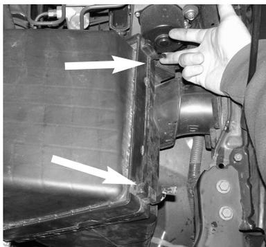
Unclip two retaining tabs holding the upper part of the air box to the lower part of the air box
