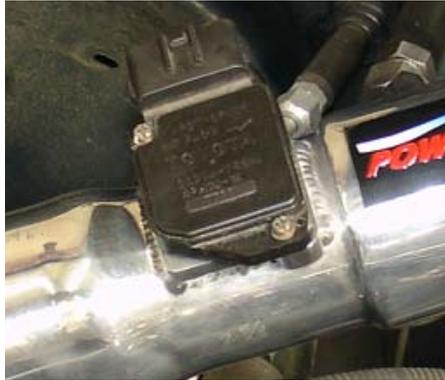
Once the mass air flow sensor has been firmly inserted into the machined sensor adapter continue to use the stock screws to fasten the sensor to the adapter.
