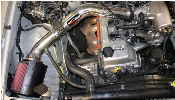
Once the intake has been installed, continue to align the entire intake for the best possible fit. Once the intake has been cleared from all objects continue to tighten all nuts, bolts and clamps. The heat-shield is now sold separately on line at "www.injenonline.com".
