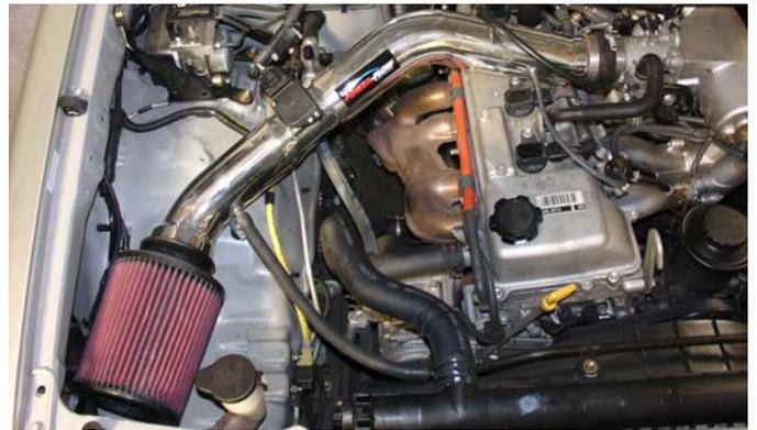
Congratulations! You have just completed the installation of the MR Tech intake system. Periodically, check the fitment of the intake system to make sure nothing has shifted or is rubbing up against anything. Regular maintenance will enhance the life of your intake system and protect you from possible voiding the warranty.
