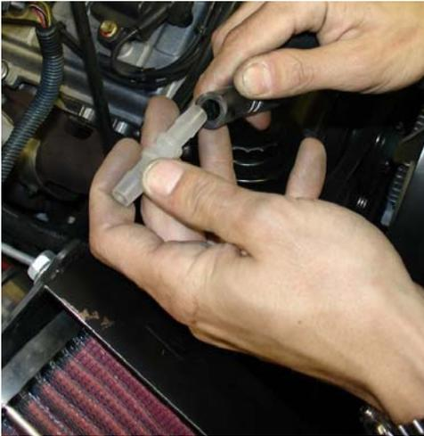
Insert the coupler provided in this kit into the stock line that comes from the Evap charcoal canister as shown above.
