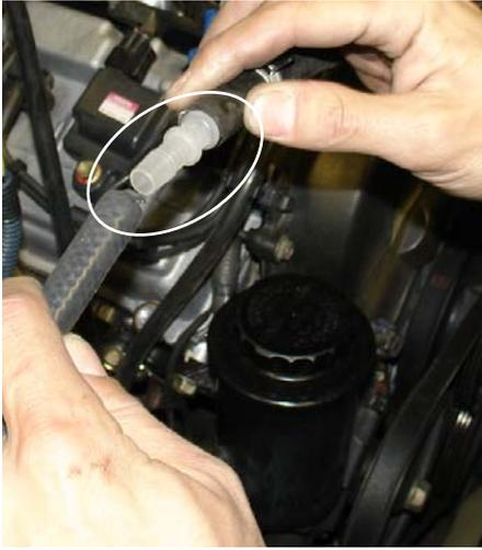
The 6" 10mm hose is pressed over the 3/8" coupler from that leads over to the Evap charcoal canister. This line is used to extend the line to allow for slack.
