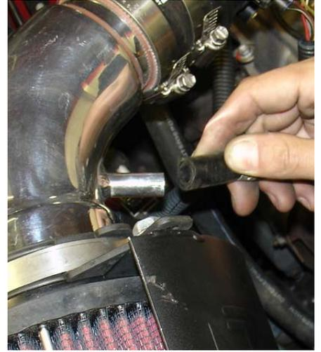
Once the 3/8" coupler and 6"-10mm hose have been installed continue to connect or press the hose over the 1/2" intake port as shown above.
