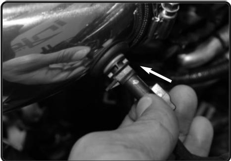
**20.** Re-install the temperature sensor to the grommet on the intake tube.
