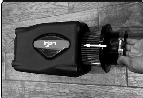
8. Install air filter to the powerflow box.
