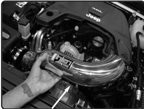
**17.** Install the intake tube to the vehicle. Position to the hose and filter.
