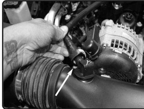
7. Pull back crank case line from air box fitting.
