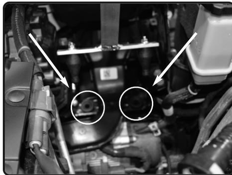
**13.** Make sure the stand off studs are seated in the OEM grommets properly.
