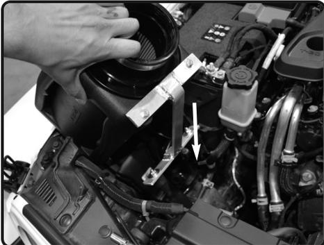
**12.** Install the powerflow box assembly into the vehicle.
