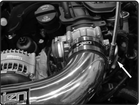
**18.** Position the intake for best fit. Tighten clamp 8mm nut driver.
