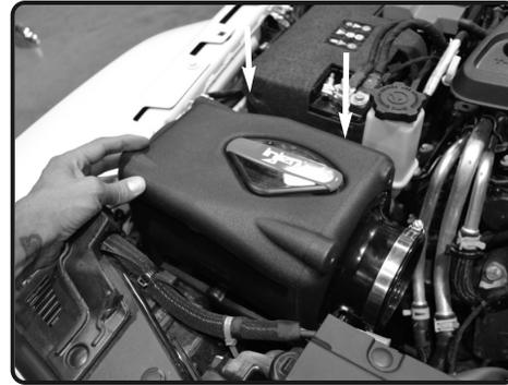
**14.** Powerflow box installed and seated properly.
