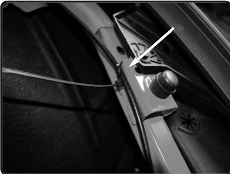
**16.** Secure the hood latch cable using provided zip tie. This will prevent the cable from hitting the filter.
