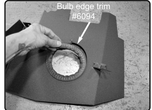
7. Install the provided Bulb edge trim to the hole cut out on heatshield. *(If trim is long, cut to length)*
