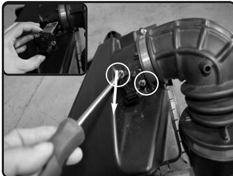
5. With T25 Torx bit, loosen and remove the 2 screws holding in the MAF sensor.
