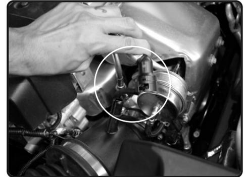
3. Now disconnect the Crank case fitting from the intake tube and pull back from tube. *Later models, see 2nd page of this instruction sheet. Tool required.*
