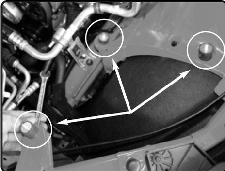
**12.** Secure all 3 vibramounts and tighten using 10mm wrench.
