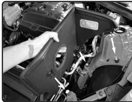
**14.** Now install the heatshield into the vehicle. Position the brackets on heat shield to the vibramounts.
