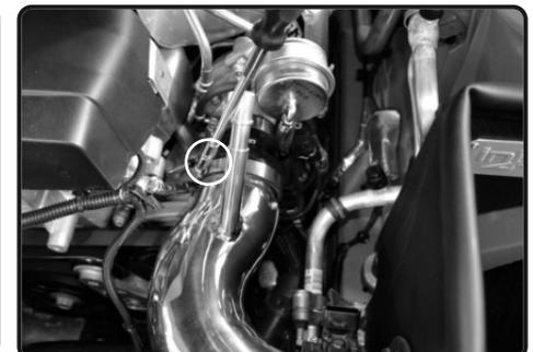
**23.** Now once positioned for best fit, tighten the clamp on step hose and secure using 8mm nut driver.
