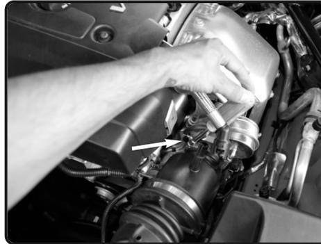
7. With 8mm nut driver, loosen the clamp on the throttle body and pull back tube from turbo.
