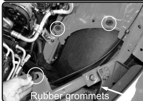
10. Remove the 3 factory rubber grommets from the stock air box location.
