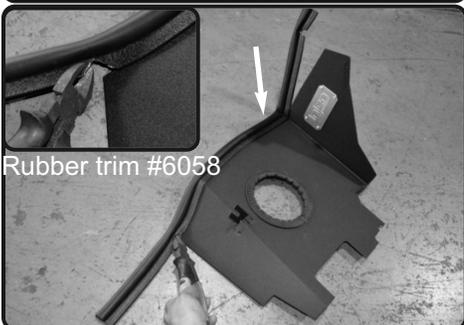
8. Now install the rubber trim to the top of heat shield. Notch corners with cutters or pliers for easier installation.
