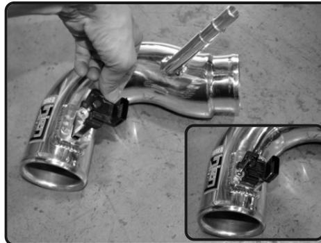
6. Now install the MAF sensor into the injection intake tube. Secure using provided M4 button head screws and tighten using 2.5mm allen key.
