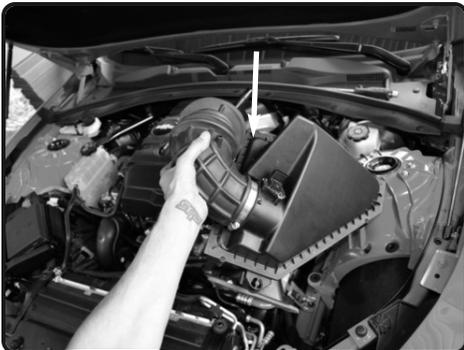
4. Now Lift up air box from vehicle and remove complete stock air box assembly.
