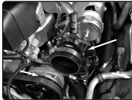
**13.** Install the provided step hose with clamps provided to the turbo. Tighten clamp on turbo only using 8mm nut driver.
