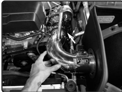
**17.** Install the intake tube to the vehicle and position the tube to the turbo and hole on heatshield. *Do not tighten the clamp.*
