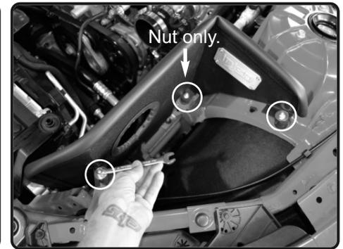
**15.** Secure the heatshield using provided fender washers and M6 nuts. *Bracket in back corner will only have nut, no fender washer.*
