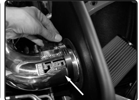
**19.** Loosen the filter clamp and install to tube first.
