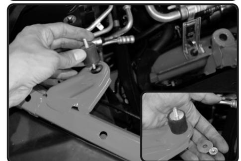
11. Now install the 3 provided vibramounts to the same holes where grommets were just removed. Center the vibramount to hole. Secure the vibramounts using provided washer and nut.
