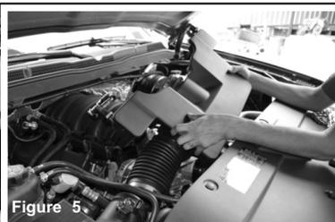
Figure 5 Remove the resonator air duct tube.
