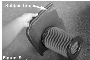
Figure 9 Place the 19" rubber trim onto the end of the heat shield.
