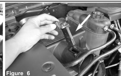
Figure 6 Disconnect the MAF sensor harness, unscrew the two screws and then pull the MAF sensor out of the OE air box assembly.
