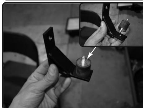
6. Now attach the vibramount to the threaded part of the bracket. Secure and tighten.
