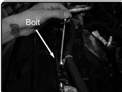
5. Locate the bolt on fender frame, loosen using 13mm wrench or socket. Save bolt for later install.
