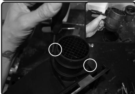
9. Loosen the 2 screws holding in the MAF sensor and remove the sensor.
