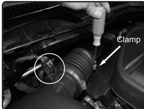
2. Loosen the clamp on the turbo housing. Disconnect MAF sensor.
