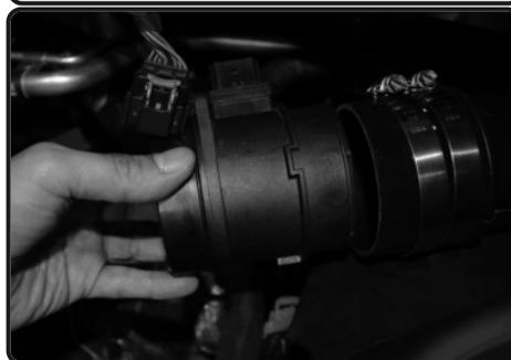
10. Install the MAF sensor to the hose. ***Make sure the arrow is going in the direction towards the turbo.***
