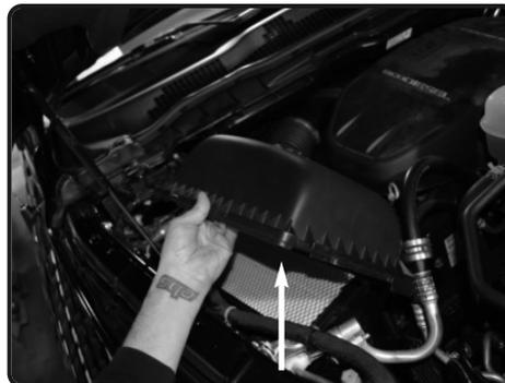
7. Carefully un-clip upper half of airbox and remove.
