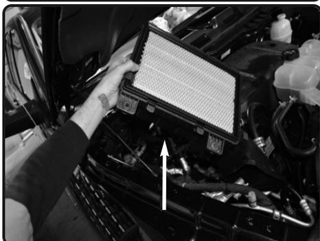
4. Lift up and remove the lower part of the air box assembly.
