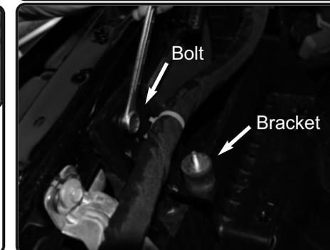
7. Now install the bracket, secure using bolt from previous step. This will be support bracket for the intake tube.
