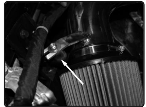
**15.** Secure the bracket using provided M6 nut and fender washer.
