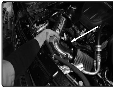
**14.** Install intake into the vehicle and position the tube to step hose and the bracket to the vibramount.
