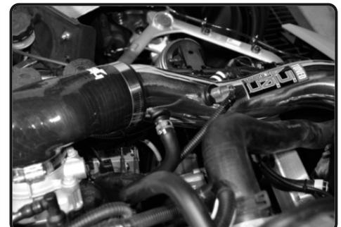
**23.** Make sure the crankcase and temperature sensor are seated and secured.
