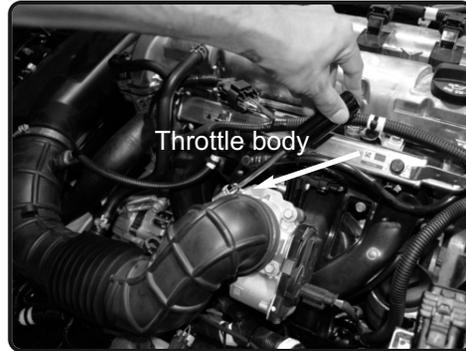
2. Loosen the clamp on the throttle body using 8mm nut driver.
