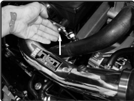
**16.** Secure the bracket using provided M6 nut and fender washer.
