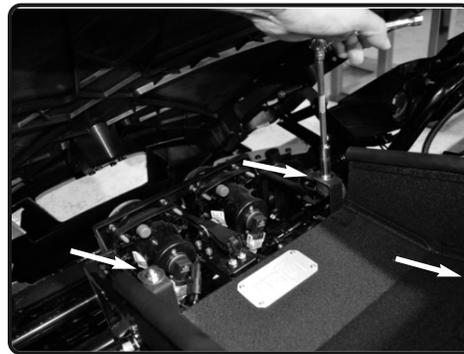
**13.** Tighten all nuts and screws using 10mm socket and ratchet.
