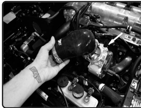
**14.** Install the cobra head to throttle body with clamps provided. Do not tighten clamps.
