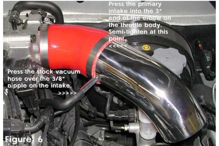
Press the primary intake into the 3" end of the elbow on the throttle body. Semi-tighten at this point.
