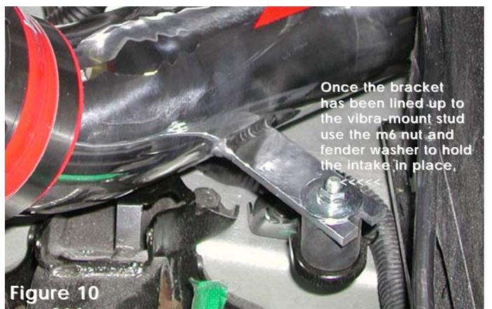
Once the bracket has been lined up to the vibra-mount stud use the m6 nut and fender washer to hold the intake in place.
