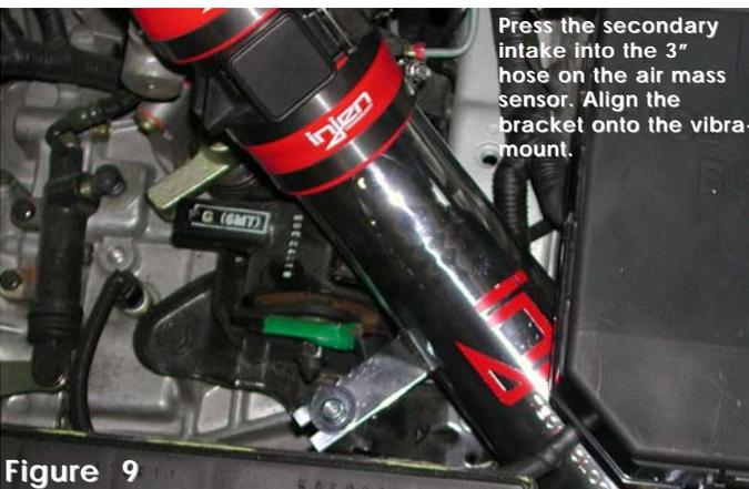
Press the secondary intake into the 3" hose on the air mass sensor. Align the bracket onto the vibra-mount.
