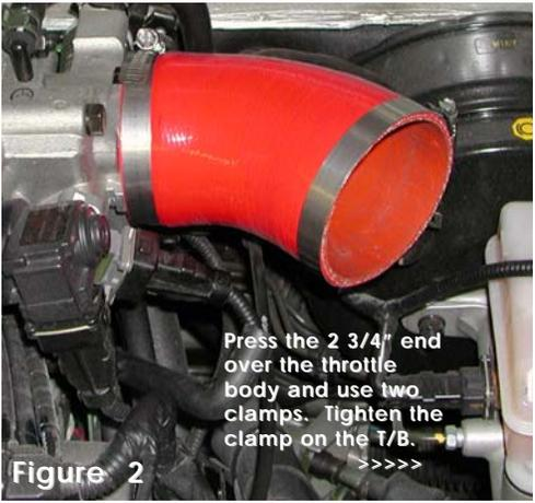
Press the 2 3/4" end over the throttle body and use two clamps. Tighten the clamp on the T/B.
