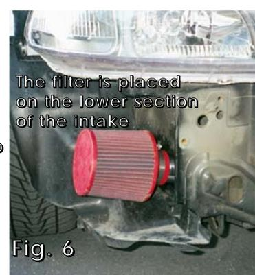
**Note: Disconnect the battery terminals before starting this installation.**
