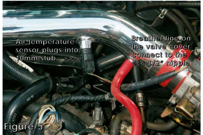
Air temperature sensor plugs into 10mm stub >>>>>
