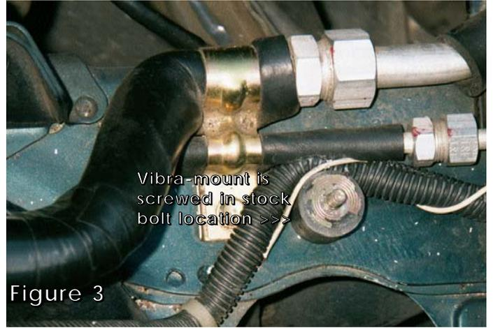
Vibra-mount is screwed in stock bolt location >>>
