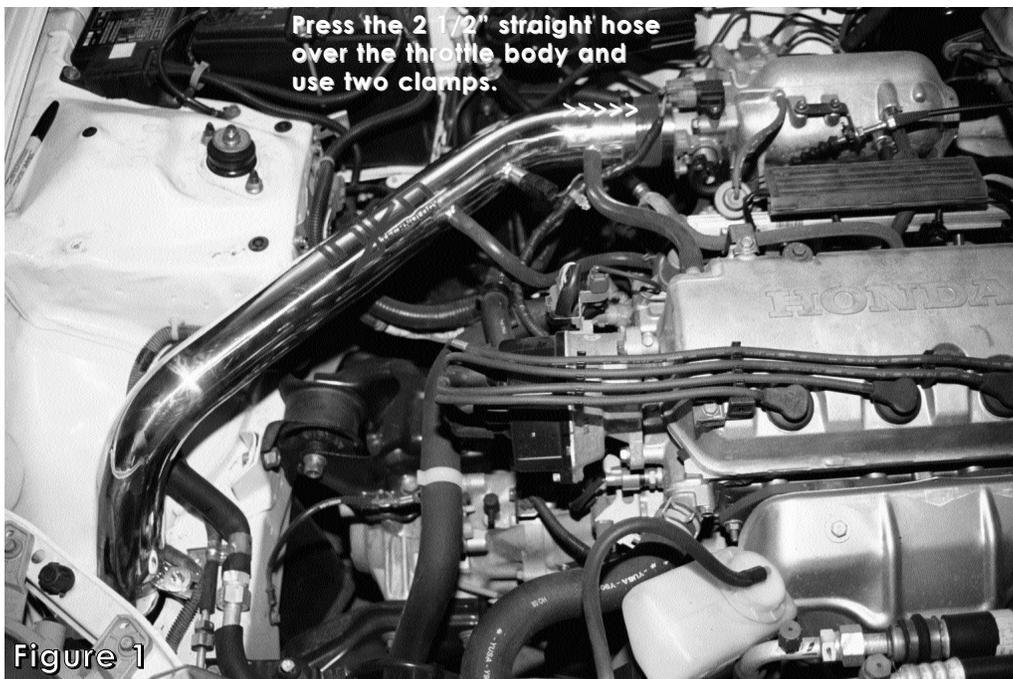
**Press the 2 1/2" straight hose over the throttle body and use two clamps.**
