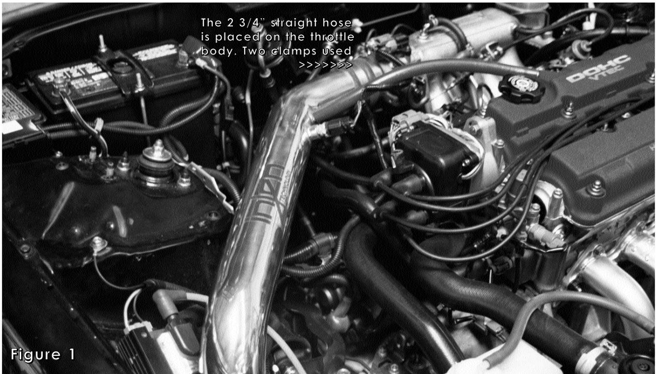
The 2 3/4" straight hose is placed on the throttle body. Two clamps used >>>>>>
