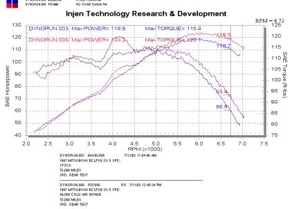
Injen Research and Development Team at work testing various intake tubing and filters. Top end showed an 8.8 horse power gain.
