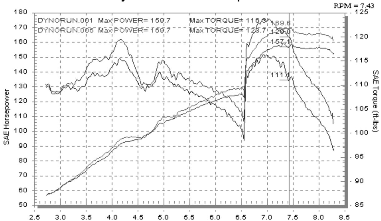
Injen Technology Research & Development Team tested its final design on Injen's own in-ground all wheel Dyno-jet. The base horse power run was 159.7 to the wheels. Injen's C.A.I increased its performance to 169.7 h/p that's an increase of 10.0 h/p gain. The peak base run came in at 157.1 while the CAI run came in at 169.6 for a total peak gain of 12.50 h/p. Torque increase was also seen through-out the band but was noticeable at top end for a total of 11.9 ft./lbs of torque.
