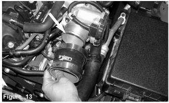
The 2 3/4" straight hose and clamps are pressed over the throttle body
