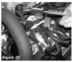
Loosen and removed the m8 bolt that fastens the charge pipe to the bracket.
