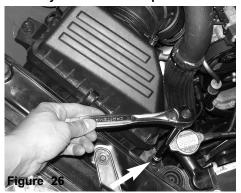
Loosen and remove the first m6 bolt located to the front of the air box cleaner.
