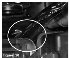
The stock tension clamp is removed and an .036 clamp is used. The intercooler piping lowered in place and pressed into the stock intercooler hose.
