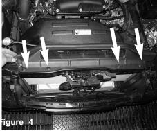
Use a phillips screwdriver to loosen and remove all four screws from the front air duct.
