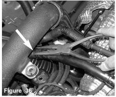
Use the needle nose pliers to compress the tension clamp on the air intake duct as shown above.
