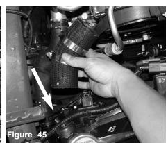
The hose off the turbo outlet is lowered into the intercooler end tank. Look for a white dot on the hose and a raised pad on the end tank, line them up.
