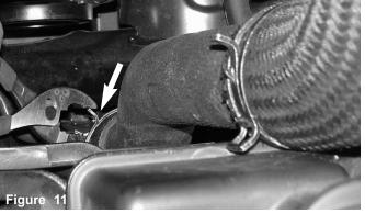
Use pliers to compress the tension clamp on lower intercooler hose. Once you have compressed the clamp slip upward away from the intercooler.
