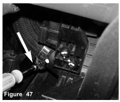
Once you have aligned the white dot on the hose and raised pad on the intercooler tank, continue to tighten the clamp.
