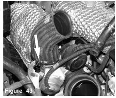
The stock hose will be removed from the turbo outlet and placed on the intercooler end tank.
