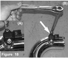
The stock bolts are used to fasten the map sensor in place (A) Use the 8mm socket to fasten the two m6 bolts over the map sensor (B).
