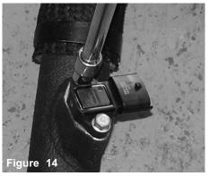
An 10mm socket is used to removed the two m6 bolts from the map sensor pad.
