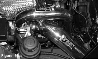
Once you have aligned intake and made sure that the length of the intake is free from any moving parts, continue to tighten all nuts, bolts and clamps. Now you are ready to reinstall the bumper, repeat steps 3-9 in reverse and re-install the front air scoop.
