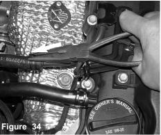
The rear crankcase hose clamp is compressed and moved forward.
