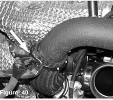
Removing charge pipe- compress the tension clamp on the hose and move back towards the hose.
