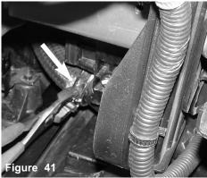
Do the same on the intercooler tank- compress tension clamp and move towards the hose, this will allow you to pull the hose off the intercooler end tank
