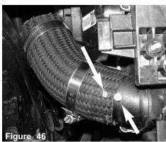
The white dot and raised pad on the end tank are lined up as the hose is pressed into the intercooler end tank. Note: the raised white pad is used as an example.
