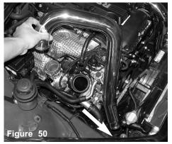
The new charge pipe is lowered into position. The lower end is lined up the the stock hose place down on the intercooler end tank.
