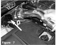
The primary intercooler piping is lower into the engine compartment. The 2 inch hose on the IC piping is pressed over the turbo inlet.
