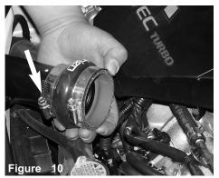
The 2 1/2" hump hose is pressed over the stock intercooler outlet pipe. The clamp on the IC pipe is tightened at this point.
