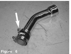
The two inch straight hose and clamps are inplaced over the primary intercooler pipe. The clamp over the pipe is tightened for now.
