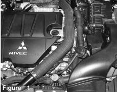
Stock upper intecooler piping to be removed.
