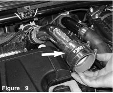
The 2 1/2" hose is aligned and pressed over the end of the primary intercooler pipe as shown above.
