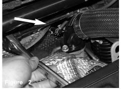
The upper intercooler piping hose is loosened at the turbo inlet as shown above.
