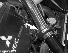
The secondary IC pipe is pressed into the 2 1/2" step hose, the other end is pressed into the 2" hose on the primary IC pipe.
