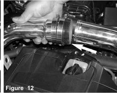
The upper secondary pipe is now pressed into the 2" hose as shown above.
