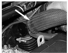
The stock intercooler hose is pulled from the turbo inlet.
