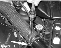
A nut driver is used to unscrew the second hose clamp at the intercooler outlet.
