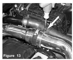
Both IC pipes are aligned for best fit, once you have aligned the primary and secondary IC pipes, continue to tighten the clamp.
