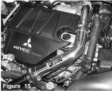
Periodically, check the fitment of the entire IC piping, shifting and rubbing of the IC piping could cause damage to the piping and other engine components.
