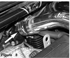
The primary intercooler pipe and hose is installed over the turbo inlet.
