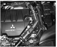
Check the alignment of the intercooler piping and all hoses and clamps then adjustments as needed.
