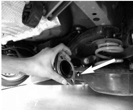
Figure 7 Install the provided gasket to the stock exhaust flange.
