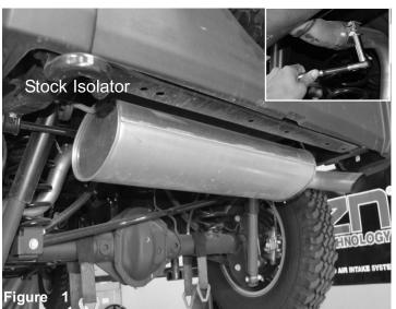
Remove the stock muffler using 15mm socket and wrench. Remove the hangars from stock isolators. Install the new Injen Axle Back Exhaust. Position the hangars to the stock isolators. Use Provided #63 torsion clamp in the kit. Position for the best to have access to the 17mm nut on clamp. **Do not tighten.** Install the Black tips to the exhaust adjust and fit to desired position and tighten.
