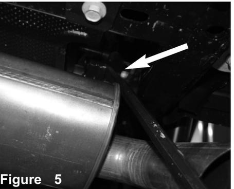
With llubrication, pull back the rubber hangars from exhaust.
