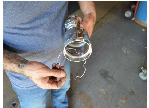
9. Install the retaining clip onto the cold side intercooler pipe.
