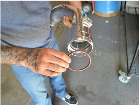
7. Install the OEM O-Ring onto the Injen cold side intercooler pipe in the same direction it was removed.
