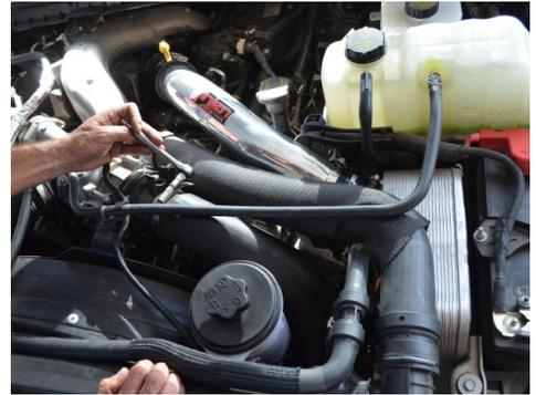
3. Loosen both clamps from the cold side intercooler pipe.
