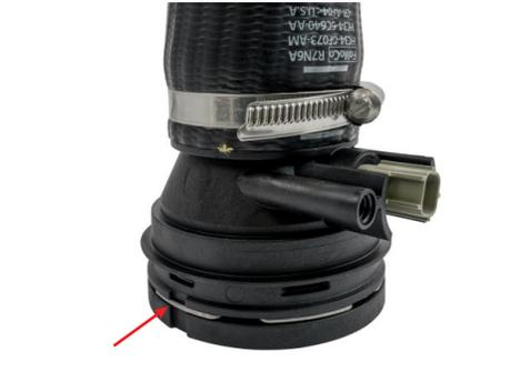
8. Remove the OEM retaining clip from the IAT sensor adapter.
