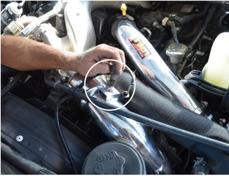
13. Install the IAT sensor onto the cold side intercooler pipe. Once fully seated, rotate the sensor to secure the tab in place.
