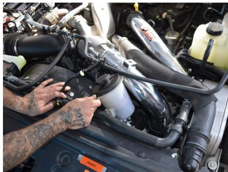
11. Remove the bolt securing the power steering reservoir then move the reservoir to give clearance for installing the intercooler pipe.
