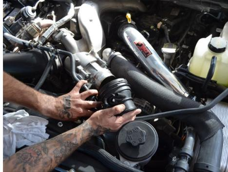
5. Disengage the retaining clip from the IAT sensor adapter then remove the adapter from the engine bay.
