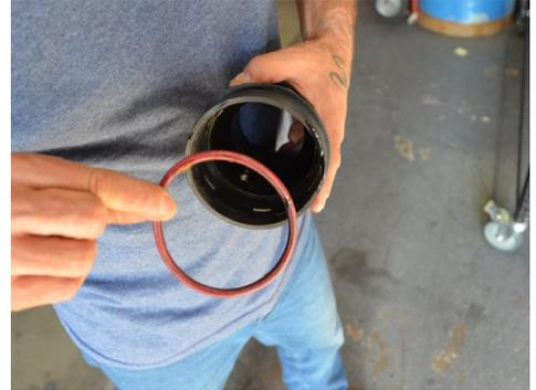
6. Remove the O-Ring from the IAT sensor adapter. Note the direction it was removed in.
