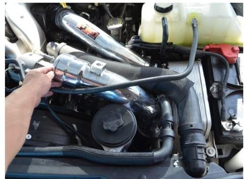
12. Once the intercooler pipe is in place. Secure the clamp then secure the power steering reservoir to its factory location.
