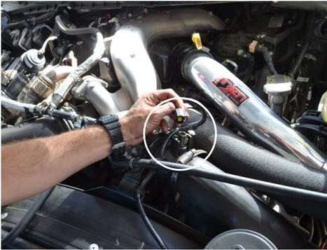
1. Disconnect the IAT sensor harness located on the OEM cold side intercooler pipe.
