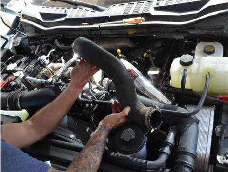
4. Remove the cold side intercooler pipe from the engine bay.
