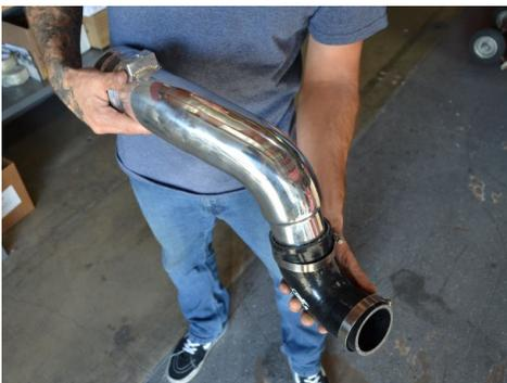
10. Install the elbow hose onto the cold side intercooler pipe. Secure using the provided clamps.
