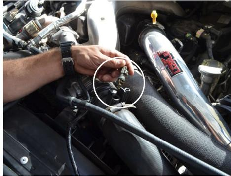
2. Lift the tab on the IAT sensor then twist the sensor a 1/4 turn to remove it from the cold side intercooler pipe.
