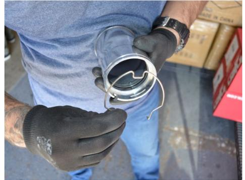
6. Install the OEM retaining clip onto the Injen secondary hot side intercooler pipe.
