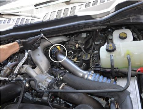
1. Loosen the clamp connecting the OEM hot side intercooler pipe to the turbo inlet.
