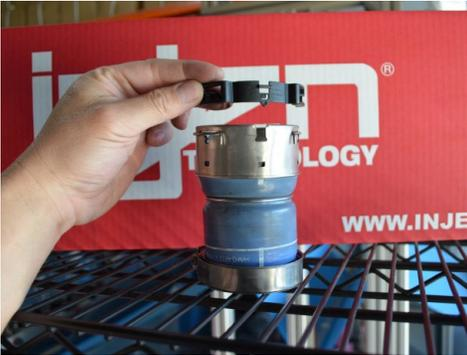
4. Remove the plastic retaining clip from the hot side turbo outlet coupler by carefully prying on both ends and then lifting up.
