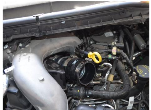
9. Install the 3.00" hump hose onto the secondary hot side intercooler pipe. Secure using the provided clamps.
