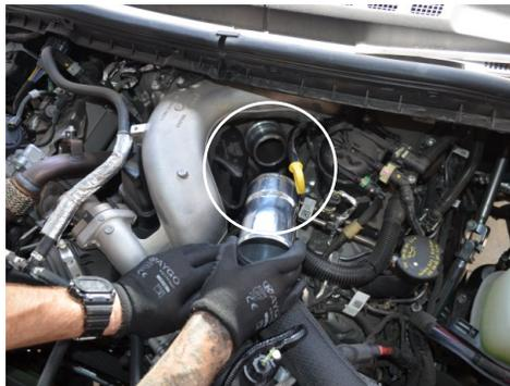
8. Install the secondary hot side intercooler pipe onto the turbo outlet. You should hear the retaining clip engage.
