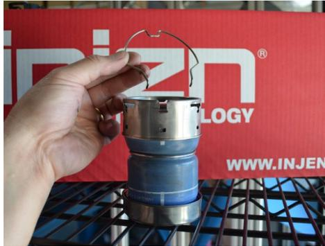
5. Remove the retaining clip from the hot side turbo outlet coupler.
