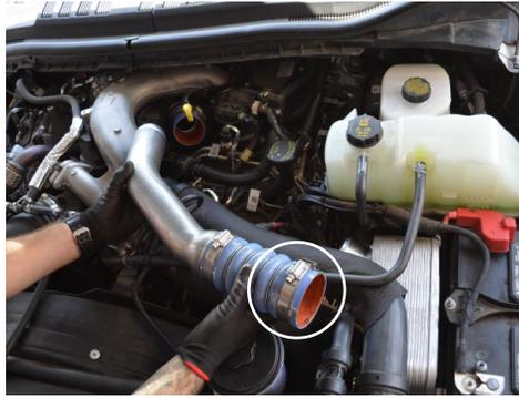
2. Loosen the clamp holding the hot side intercooler pipe to the intercooler then remove the hot side charge pipe.
