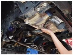
2. Insert the hanger to the rubber insulator then connect the muffler delete pipe to the mid pipe.
