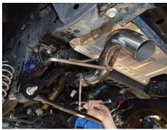
3. Secure the muffler delete pipe using the OEM clamp.
