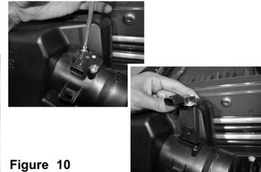
**Figure 9:** **Figure A:** Loosen the 2 screws holding in the MAF sensor. **Figure B:** Now lift up the MAF sensor and remove.
