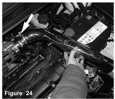
The primary intake is now lowered into the engine compartment. The upper intake is inserted into the throttle body hose.
