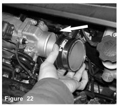
Thefirst 2 3/4" straight hose is aligned to the throttle body as shown above.
