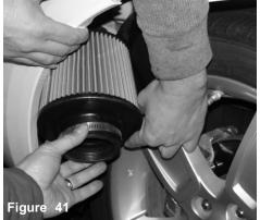
The filter is now inserted into the driver side corner bumper, the filter neck is aligned to the intake.
