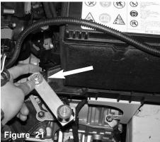
The bracket assembly is lowered into the engine compartment. The M6 bolt and washer are used to secure bracket to the air box mounting brace.
