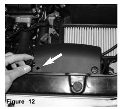
Once you have loosened the center screw on the clip, continue to pull the clips out.
