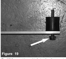
The M6 flange nut is used to fasten the vibra-mount to the aluminum bracket.
