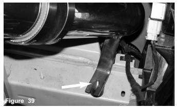
The secondary intake bracket is aligned to the vibra-mount stud.
