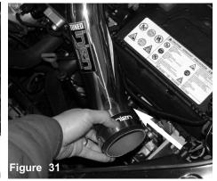
Converting the intake into a cold air intake, aligned and slip the 2 3/4" hose over the end of the intake.
