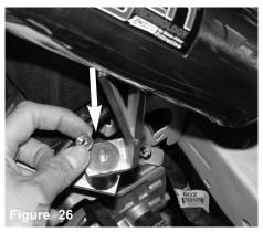
The intake bracket is now secured with an m6 flange nut and washer.
