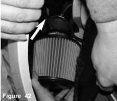
The filter is pressed over the end of the intake as shown above
