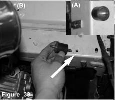
The vibra-mount is aligned to the top frame in the engine compartment (A). The vibra-mount si installed and screwed in place (B).
