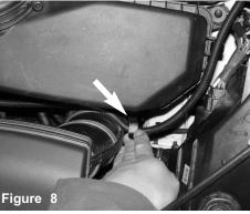
Unlatch the two clips holding the upper air box to the lower box. The first metal clip is unlatched.
