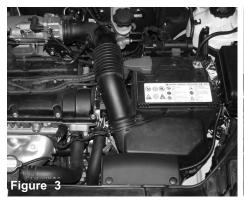
Stock air intake cleaner and air ducts shown in this picture. Before getting started with the installation, disconnect the negative battery terminal.
