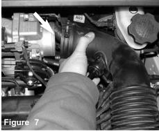
Once you have loosened the clamp, continue to detach the air duct from the throttle body.
