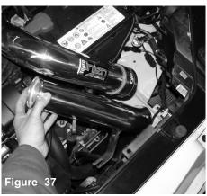
The secondary intake is now lowered into the driver side corner bumper.
