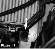
The third bolt is loosened and removed from the lower air box.
