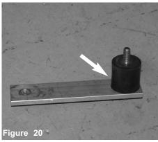
The vibra-mount is now attached to the bracket.
