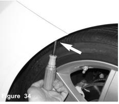
The bumper corner screw is loosned and removed in the wheel well.
