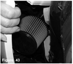
Once the filter stops come to rest over the intake end, continue to tightened the filter neck.
