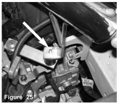
As the upper intake is inserted into the throttle body hose, The intake bracket is aligned to the vibramount stud.
