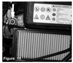
The second bolt is loosened and removed from the lower air box.
