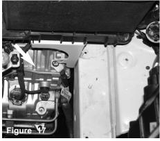
The lower air box and panel filter has now been removed from the engine compartment.
