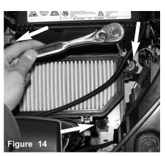
The first of three bolts are loosened from the lower air box as shown above.
