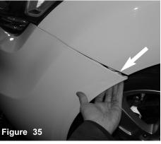
Once the screw has been removed, continue to pull back and the drive side corner bumper.
