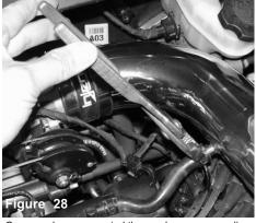
Once you have connected the crankcase vacuum line, continue to slide the tension clamp over the end of hose..
