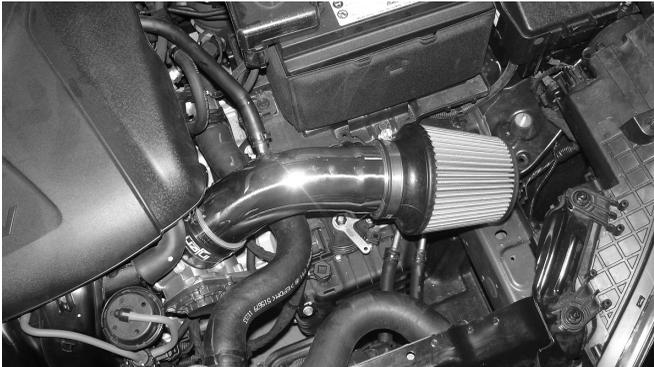
This intake system can be converted short ram for emergency situations.
