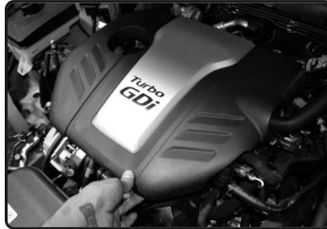
**25.** Re-install the engine cover and secure.
