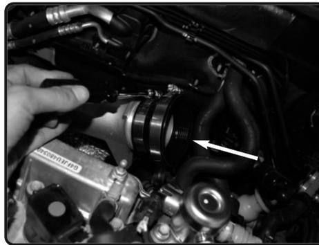
**14.** Now install the step hose with clamps provided to the turbo housing. Tighten the clamp on turbo housing only.
