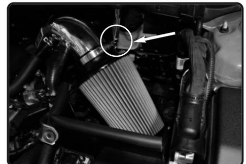
**23.** Install the air filter to the intake tube and tighten using 8mm nut driver.
