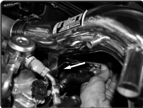
**16.** Now secure the bracket using M6 nut and fender washer.
