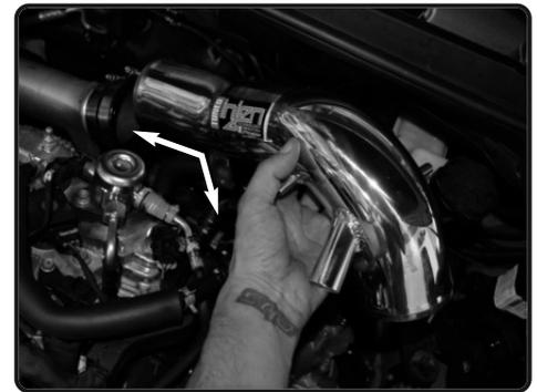
**15.** Now install the intake tube into the vehicle. Position the bracket on the tube to the vibramount. And the tube to the step hose.
