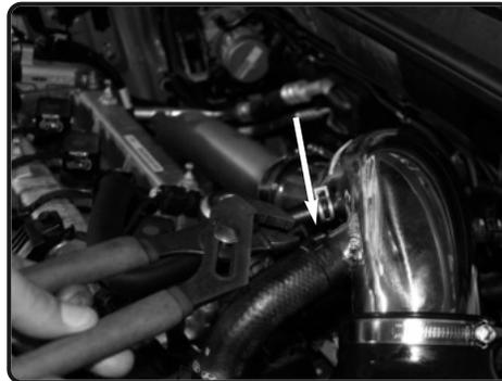
**18.** Connect the BOV line to the intake tube fitting and secure.
