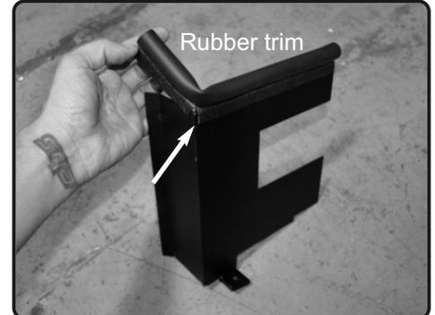
**19.** Install the provided rubber trim, to the top of the heatshield. Notch corner with pliers or cutters for easy install.
