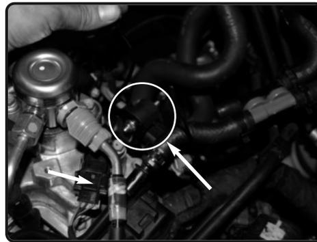
**13.** Now secure the vibramount using M6 nut. Secure and tighten using 10mm socket or wrench.
