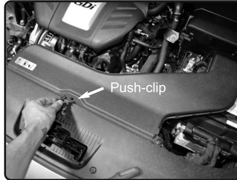
2. Disconnect the push clips from the factory scoop.
