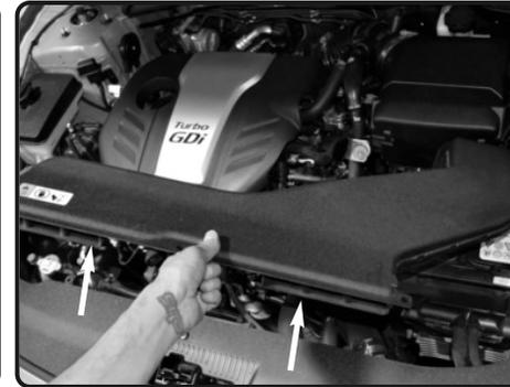
7. Now lift up and remove the factory scoop.
