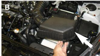
4. **Figure A:** Unclip the two tabs from the lower air box assembly to the upper air box assembly. **Figure B:** Detach the upper air box assembly from the lower assembly.
