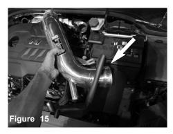
Install the intake tube through the heatshield and install the assembly into the vehicle.
