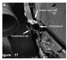
Make sure the vibramount secures the heatshield and is also used for the bracket on the intake tube. Position for best fit.
