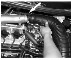
Use a 10mm socket and rachet and loosen the 10mm clamp bolt on the air duct located on the Turbo charger compressure outlet. Pull the air duct from the outlet.
