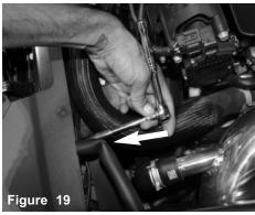
Secure the front of the heatshield to the OEM location from step 12. Secure using original screw.
