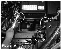
Use a 10mm socket, rachet and extension to remove the three 10mm bolts on the lower air box assembly indicated by the arrow. Save 1 bolt for later install.
