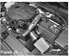
Reinstall the engine cover. Your intake installation is now complete. Go over all your clamps and fittings to make sure they are snug. Check the clearance on the pipe and make sure it does not make contact with any components in the engine bay.
