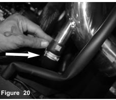
Install and secure the diverter valve to the fitting on the intake tube..
