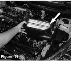
Now the lower air box assembly can be removed from the engine bay.
