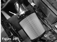
Install the filter to the intake tube and secure using 8mm nut driver.
