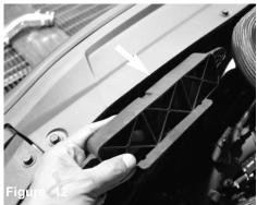
Loosen the 2 bolts holding in the front scoop vent and remove. Save 1 screw for later install.
