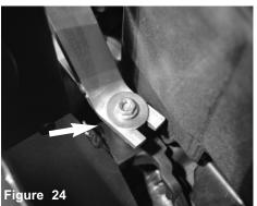
With provided M6 nut and fender washer, secure the bracket.
