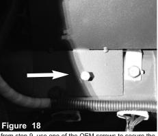
from step 9, use one of the OEM screws to secure the bottom of the heatshield.
