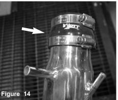
Install the step hose with clamps to the intake tube.
