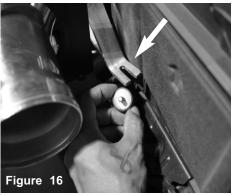
Secure the tabe on heatshield using the M6 vibramount.
