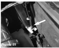
Tighten the bracket using 10mm socket or wrench
