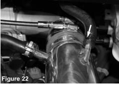
Position the intake and tighten the clamp on the turbo side
