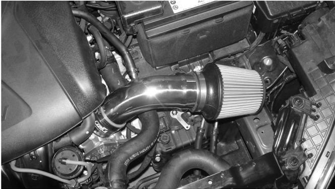
Check the entire air intake system for best possible fit, once proper clearance has been made through out the length of the intake, continue to tighten all nuts, bolts and clamps. *Short Ram image shown above.*
