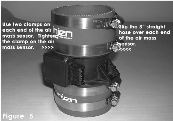
Use two clamps on each end of the air mass sensor. Tighten the clamp on the air mass sensor. >>>>
