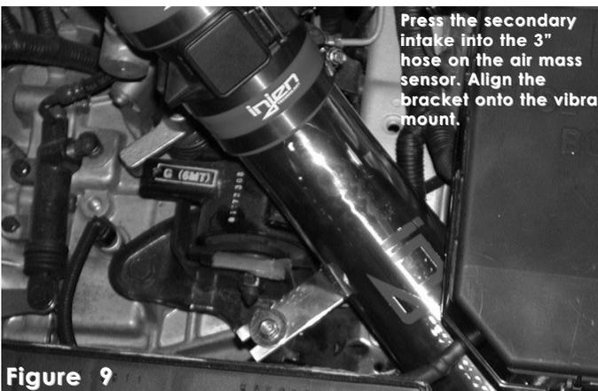
Press the secondary intake into the 3" hose on the air mass sensor. Align the bracket onto the vibra-mount.
