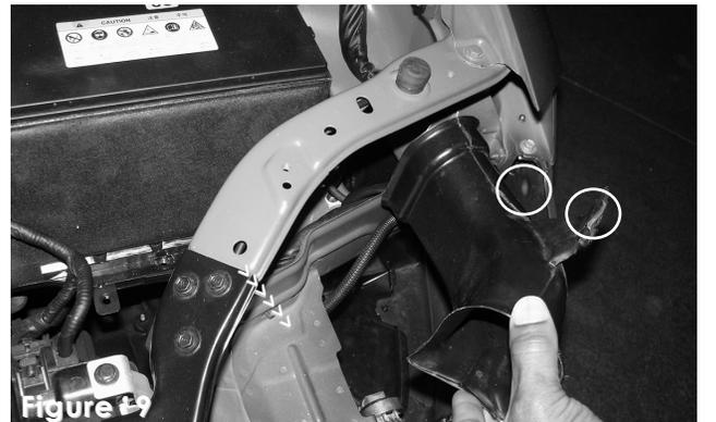
Remove plastic clips or bolts from the air intake duct connected to the fender well. Once fasteners have been removed, continue to remove the plastic air duct from the fender well.
