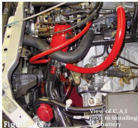
**Note: Removal of the entire battery and battery tray will be required for this installation.**
