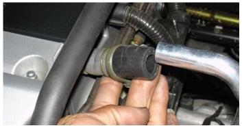
Take the stock crankcase hose and press it over the large port on the intake. Press it until you get the best fit on the intake and the bracket is setting flush on the vibra-mount.
