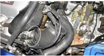
With the specially molded 60 degree elbow, press the 2 7/8" side over the throttle body. Press the elbow over the throttle body until the edge butts up against the velocity stock inside of the molded elbow. Position the elbow and semi-tighten the clamp on the throttle body side.
