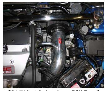
SP1476 installed on Acura RSX-Type S
