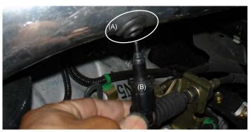
Press the 1525 grommet into the pre-drilled hole on the intake (A). Once the grommet has been properly set in place take the air temperature sensor and press it into the grommet. (B).
