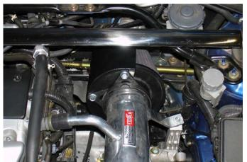
Shot of the HS3500 installed on the intake. Wrinkle black coating is highly resistant to heat and deflects heat that comes in direct contact to the filter.
