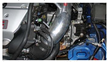
Once assembled, press the opposite end of the MR Tech intake into the three inch opening of the molded elbow.
