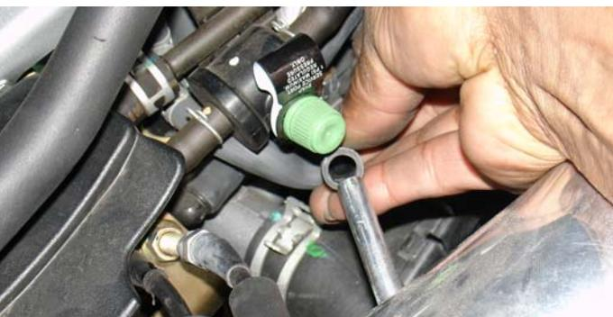
Take the small vacuum port and press it over the long 3/8" port on the intake. Make sure the vacuum hose is secured.
