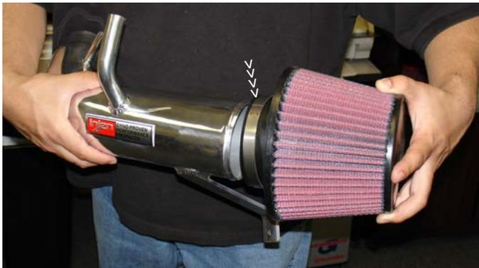
Take the new 3 1/2" neck filter and press it over the Mega-Ram Tech intake. Press until the inside velocity stack in the filter butts up to the end on the intake. Once the intake has been positioned in the correct place, continue to fasten the clamp on the filter now.
