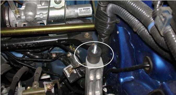
Once the stock air intake box and duct has been removed from the engine compartment, take the vibra-mount and fasten it to the pre-tapped brace. Be sure to screw the vibra-mount into the brace until it bottoms out.
