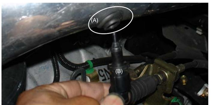
Press the 1525 grommet into the pre-drilled hole on the intake (A). Once the grommet has been properly set in place take the air temperature sensor and press it into the grommet. (B).
