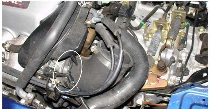
With the specially molded 60 degree elbow, press the 2 7/8" side over the throttle body. Press the elbow over the throttle body until the edge butts up against the velocity stock inside of the molded elbow. Position the elbow and semi-tighten the clamp on the throttle body side.
