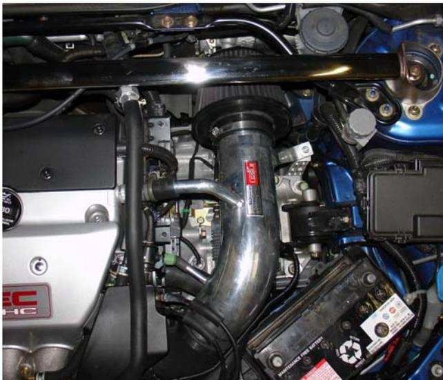
**SP1476 installed on Acura RSX-Type S**
