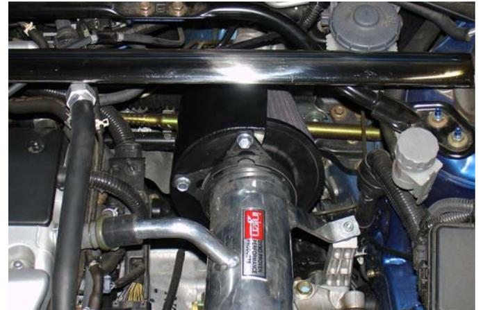
Shot of the HS3500 installed on the intake. Wrinkle black coating is highly resistant to heat and deflects heat that comes in direct contact to the filter.
