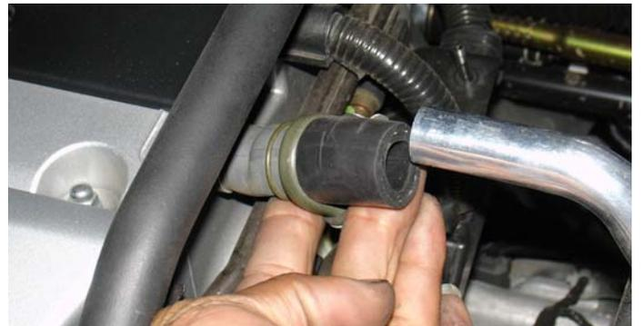
Take the stock crankcase hose and press it over the large port on the intake. Press it until you get the best fit on the intake and the bracket is setting flush on the vibra-mount.
