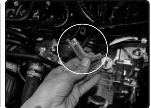
7. Remove the bracket from the vehicle. Save screw for later install.
