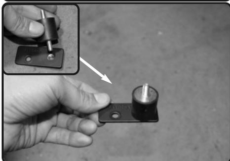
8. Now install the M6 vibramount to the threaded fitting on the provided bracket. Secure and tighten.
