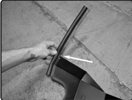
**12.** Now install the rubber trim to the heatshield. Cut a notch in corner for easier installation.
