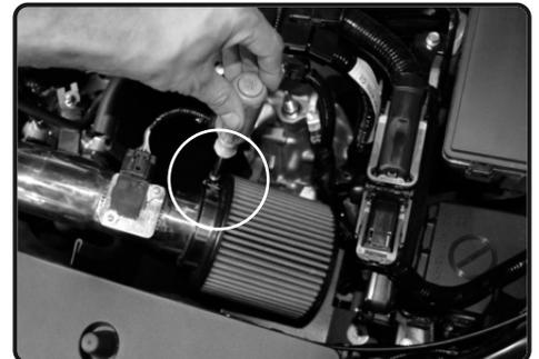
**23.** Install the filter and tighten clamp using 8mm nut driver.
