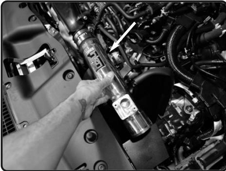
**17.** Install the intake tube and position the tube to straight hose and bracket to vibramount.
