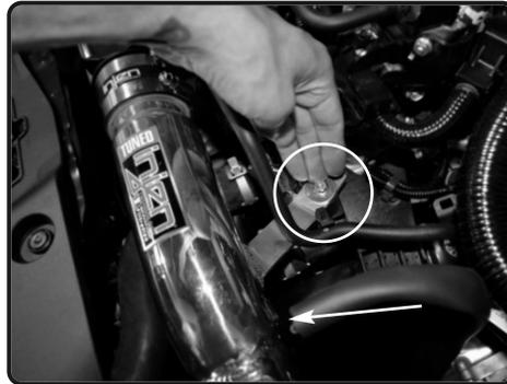
**18.** Secure the vibramount using provided M6 nut and fender washer, tighten using 10mm socket and fender washer.
