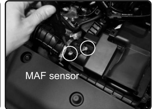
3. Using phillips screwdriver, loosen the 2 screws holding in the MAF sensor.
