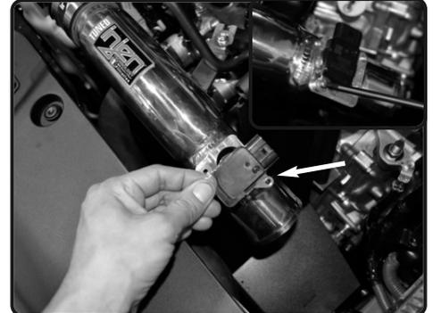
**19.** Install the MAF sensor into the intake tube. Secure using factory screws and tighten.
