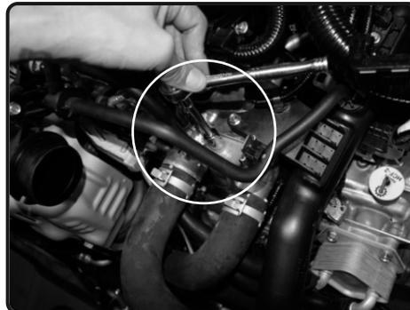
6. Locate the bracket on the engine holding in line. Pull back harness and loosen the bracket using 10mm socket or wrench.
