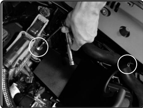
**16.** Secure and tighten both screws using 10mm socket or wrench on heatshield.
