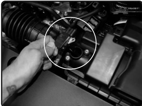
4. Remove the sensor from the air box. Save screws for later install.
