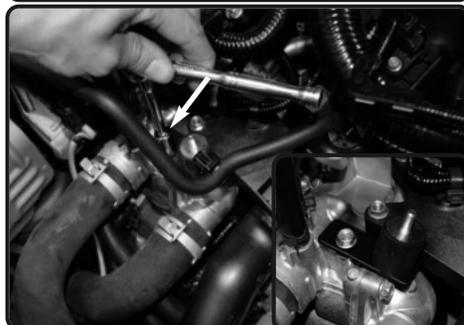
9. Now install the new provided bracket to the engine, secure using the original screw. Tighten using 10mm socket or wrench.
