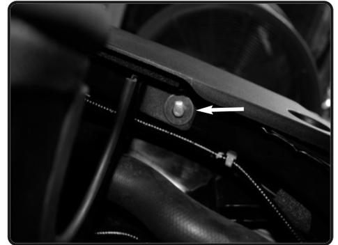
**15.** Secure the tab to the front of the radiator support. Locate the threaded insert and secure using provided M6 screw and fender washer.
