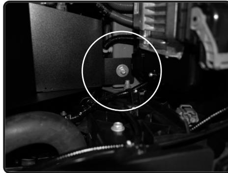
**14.** Secure the bottom of the heatshield to the threaded insert on vehicle frame using provided M6 screw with fender washer.
