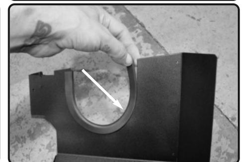
11. Install the vinyl trim to the hole cut out on heatshield.
