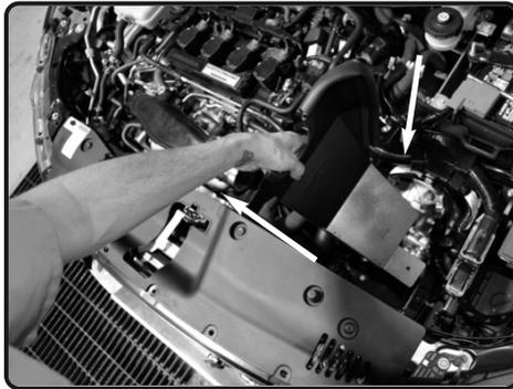
**13.** Install the heatshield into the vehicle and position.
