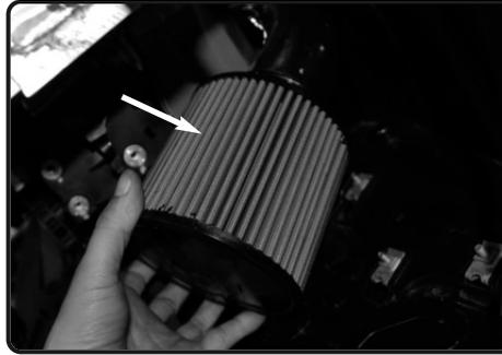
**26.** Install the filter to the lower intake tube and secure using 8mm nut driver.
