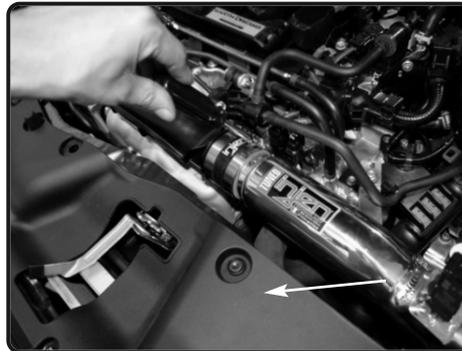
**18.** Tighten the clamp on straight hose.
