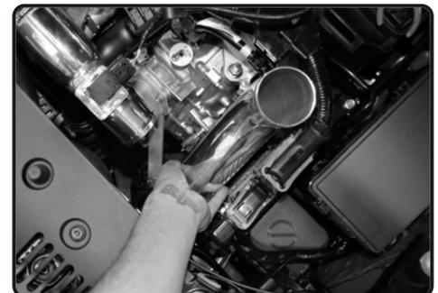
**23.** Install the lower intake tube assembly. Position the tube to upper intake tube and bracket to the vibramount.
