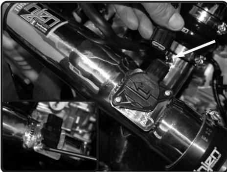
**16.** Install the MAF sensor into the machined pad. Secure using 2 two screws from step 4.
