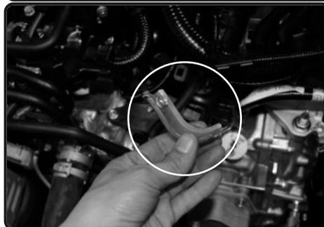
10. Remove the bracket from the vehicle. Save screw for later install.
