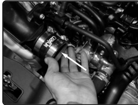
**13.** Install the 2-3/8" straight hose with clamps to the turbo housing. Tighten the clamp on the housing only.
