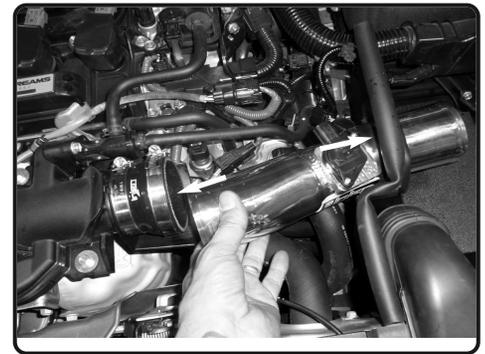
**15.** Install the intake tube assembly into the vehicle through heatshield and position.
