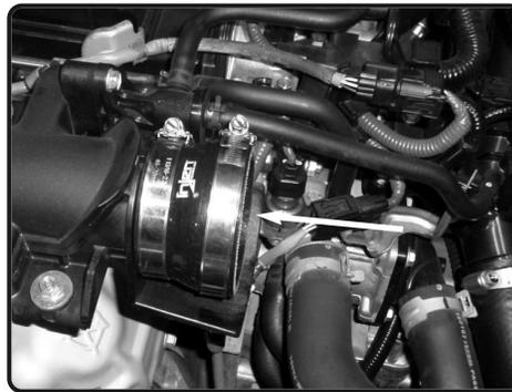
**14.** Attach the hose with clamps to the intake tube.
