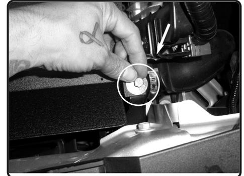
**19.** Secure the side of heatshield using provided M6 fender washer and screw. Secure and tighten.
