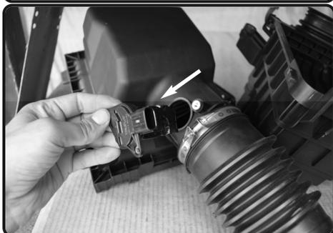
8. Loosen the 2 screws holding in the MAF sensor and remove. Save screws for later install.
