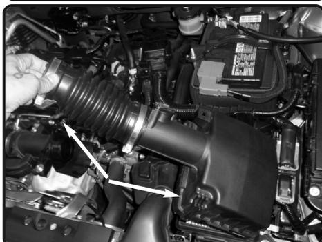
5. Now un-clip the upper part of the air box assembly. Lift up and remove from the vehicle.
