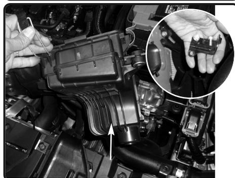
6. Carefully lift up corner of air box, this will require some force. Remove the bottom half of the air box out of vehicle. Loosen the 2 bolts holding in the air box bracket and remove bracket. Save bolts for later install.
