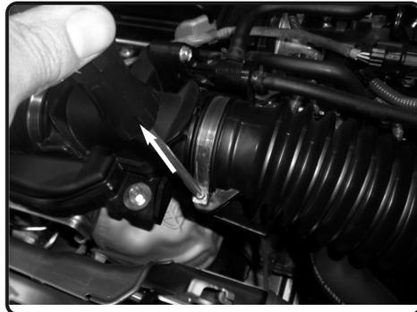
2. Loosen the clamp on the throttle body using phillips screwdriver or 5.5mm socket or screw.
