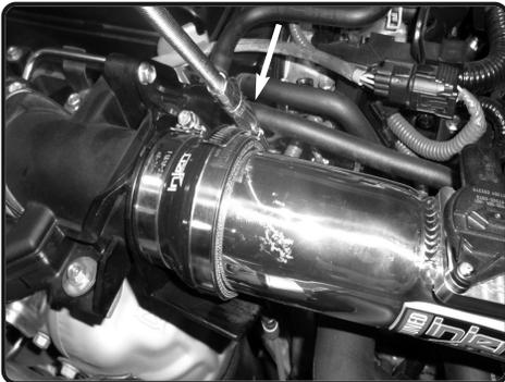
**16.** Rotate and position. Tighten all clamps using 8mm nut driver.
