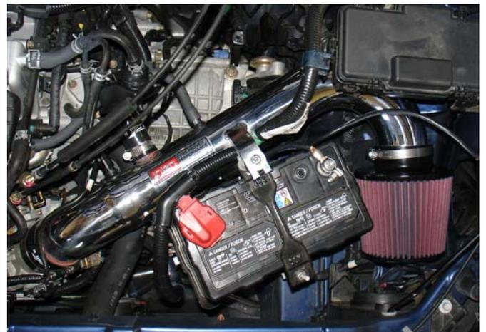
**Prior to starting this installation, disconnect the negative battery terminal.**
